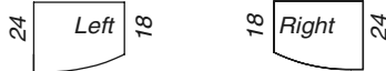
Bridge top AO uses the 18" deep end to connect to the S50-CNR-__18 corner top
